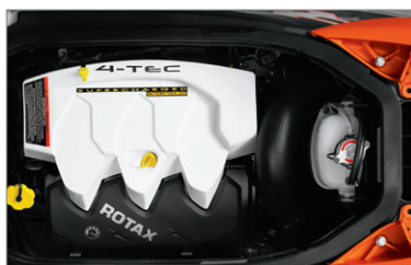
255 hp Rotax 4-TEC engine
