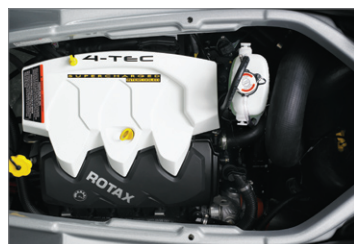
255 hp Rotax 4-TEC engine
