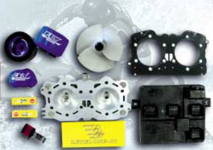
(Right) All that's included in the Level One package for the Sea-Doo: the reprogramming of your craft's MPEM, Fly Racing Flame Arrestors, air filter and a NuJet impeller. It's simple but effective.
